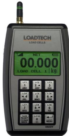
The LTW620 consists of 2 parts. The load cell and a hand held unit. The load cell amplifier is built into the load cell and contains precision circuitry which amplifies and digitizes the load cell signal and then transmits it via a radio signal to the hand held receiver.
