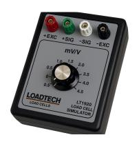
The LT1920 is a portable load cell simulator that generates fixed calibrated mV/V output step signals that can be used to test, troubleshoot and calibrate load cell installations. The LT1920 has an equivalent bridge impedance of 350Ohms and can generate a mV/V output signal between -0.5 and +4.5mV/V.
