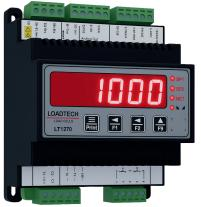
The LT1270 DIN rail mount load cell indicator is a high-precision digital device designed for load cell and strain gauge applications. Key features include:
