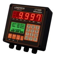
The LT1320 Belt Weigher indicator is a precision digital indicator for belt weighing applications. The LT1320 takes the weight and speed information from a belt conveyor system to accurately calculate rate and total material transferred.
