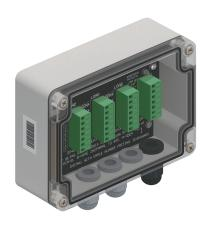
The load cell junction / summation box allows for easy connection / summation of up to 4 load cells to be connected in parallel to the load cell instrumentation. Features of the junction / summation box include an IP65 protection rating,
