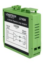
The LT1820 adopts unique electromagnetism isolation to achieve high accuracy and linearity. It can drive up to 300 ohms and boasts an isolation voltage of >3kV. The main use for a 4-20mA loop isolator is for the elimination of ground loop measurement problems.
