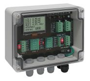
The SMART load cell junction / summation box allows for easy connection / summation of 1 to 4 load cells to be connected in parallel to the host load cell instrumentation. The smart junction box continuously monitors each individual load cell as well the excitation voltage. A relay output is de-energised if any of the listed below alarm conditions are met or if power to the SMART junction box is off. The SMART junction box can be powered from the host weighing instruments
